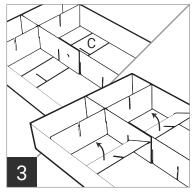
slide another Part C under Part D, then tilt it up into position. You will have to slightly lift the long divider (D) to position the short dividers (C) completely into place. Repeat this process for the remaining short dividers.
