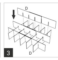
Assemble all dividers, using the three longer dividers made in step 2 as the long vertical dividers.
