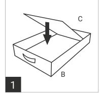
Insert the two bases (Part C) into each of the two trays (Part B).
