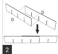
Overlap the first notch in two dividers (Part D) to create longer vertical dividers.
